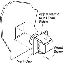
Figure 13 - Installing Horizontal Vent Cap
